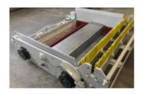
The unique KVM filling system is based on utilizing the correct type of filling box and controlling the amount of concrete delivered into the filling box. This ensures a precise filling and uniform product density, height and surface quality.
