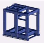
isolated from the main frame by isolation the vibrations.
