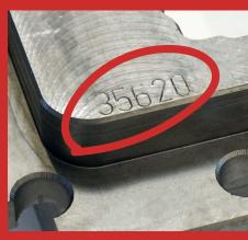
Each insert has its own unique and traceable number. In addition, a sample piece from the insert is always kept at KVM.
