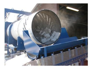
KVM Inline Tumbling Systems are adapted to handle products only 24 hours old. The systems can tumble and cube the volume from the smallest block machine to the massive flow of products from a big board KVM block machine with a capacity of more than 375 m2 per hour.
