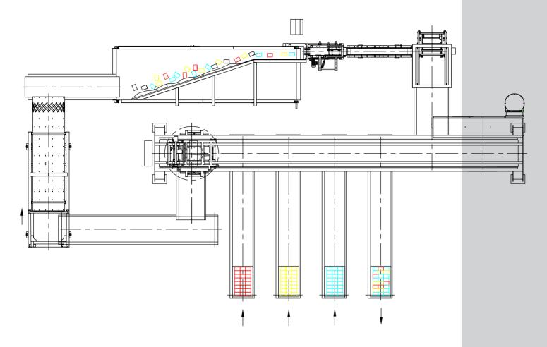
The KVM off-line system is used by producers with the highest demands for quality and flexibility. The off-line system gives the possibility for mixing pavers with up to four different colours with customer adapted variations.
