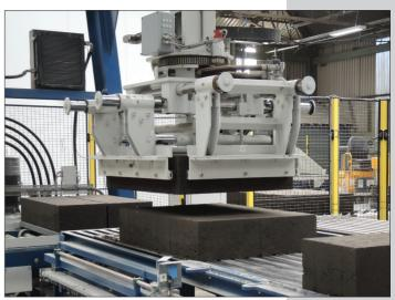
The KVM cubers are constructed for maximum versatility, and can handle all products produced on a blockmachine. The KVM cubing systems are characterised by long life, short cycle time and great reliability.
